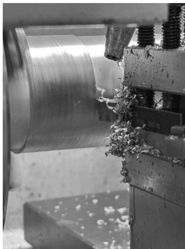
Fig. 3 Machining of the cast of the AlSi7Mg0.3 alloy
