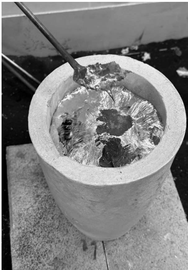
Fig. 1 Oxide layer removal before casting
