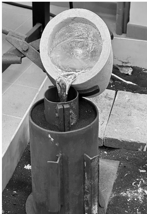
Fig. 2 Casting of pure AlSi7Mg0.3 alloy
