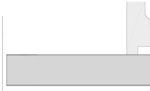
Fig. 7 Model imperfections arising in the creation of the midsurfaces
