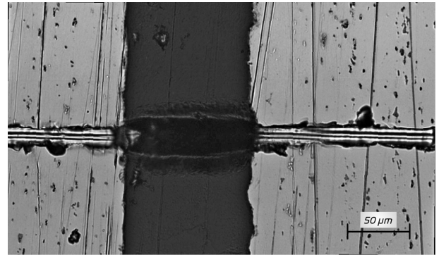
Fig. 2 Microscopic photo of a nanoscratch on an adhesive bond made with 0.1\text{ mm} thick E57/PAC adhesive material
