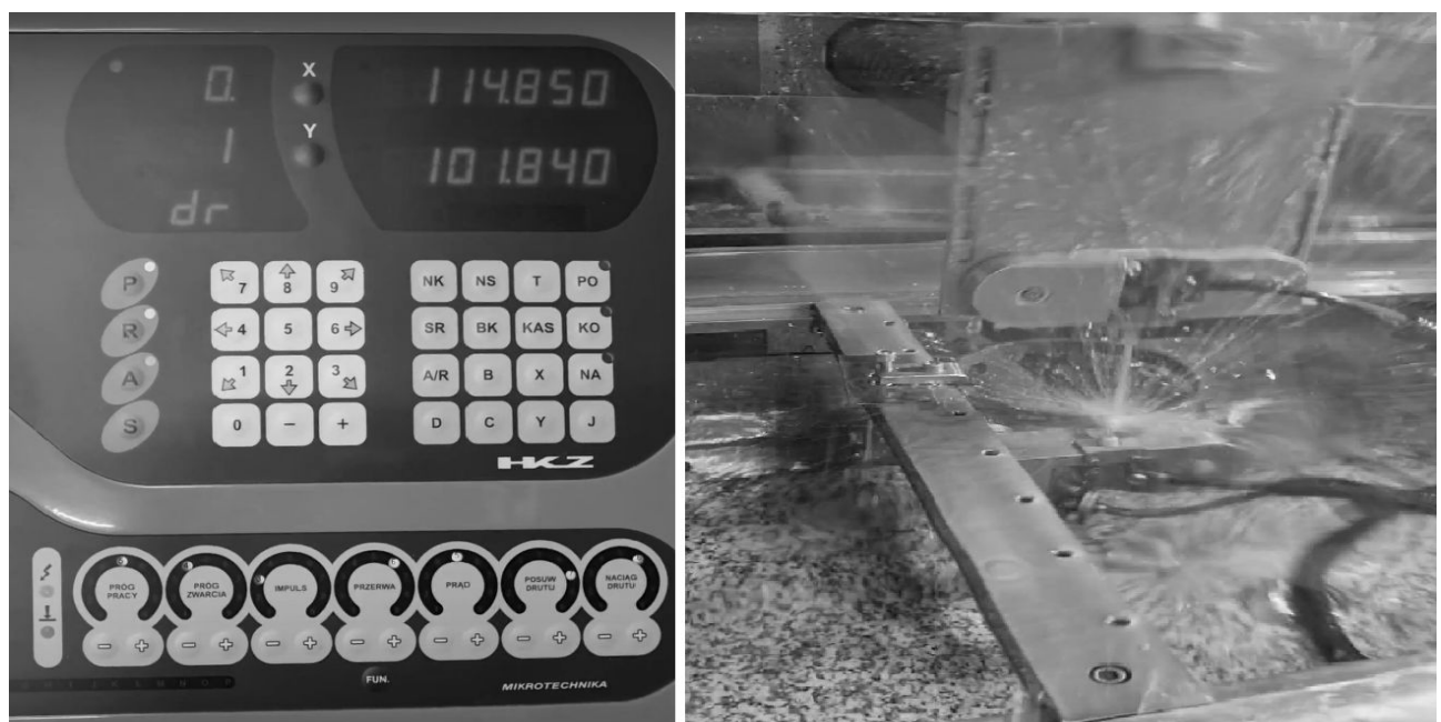
Fig. 1 Wire electrical discharge machine ZAP BP 800— parameter control panel and cutting area
