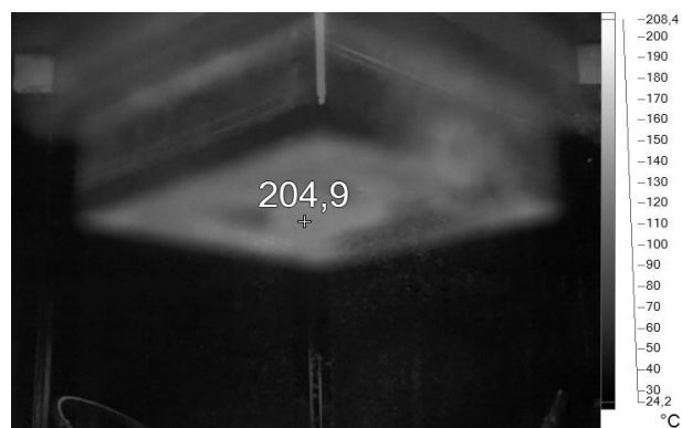
Fig. 9 Temperature reading before commencing automatic forging for the upper die
