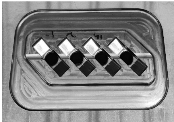
Fig. 5 View of the single cavity for the slide block in the lower die for manual forging process
