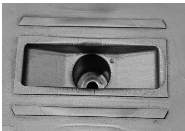
Fig. 6 View of the multi-cavity for the slide blocks in the lower die for automatic forging process
