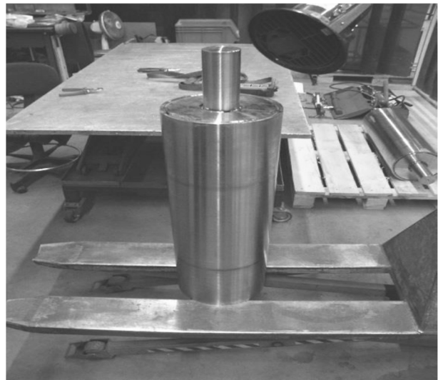
Fig. 3 Preparation of the butt weld before the welding operation
