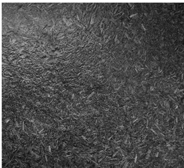
Fig. 2 Surface appearance of composite made from ground benzoylated DP stems
