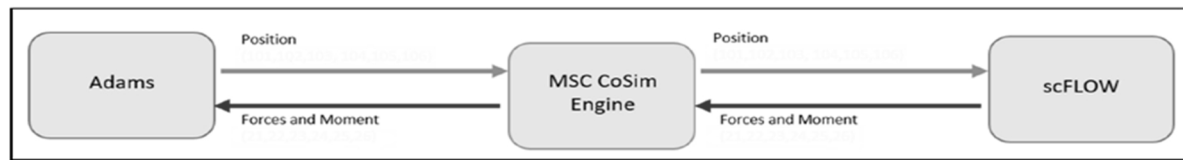
Fig. 9 MBS and CFD cosimulation scheme [author]
