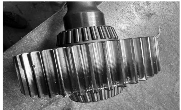
Fig. 14 A photo of the z_1 (large) gear after the load test
