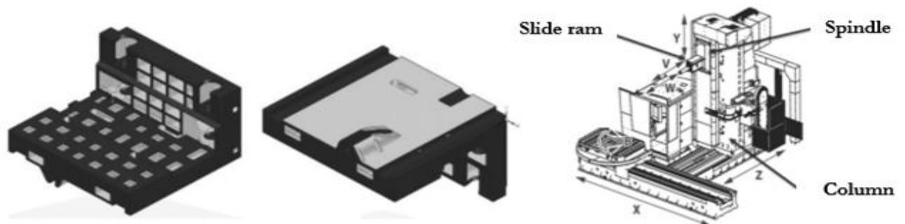
Fig. 1 Cast iron spindle with globular graphite and diagram of horizontal boring machine WHR 13 with spindle marking
