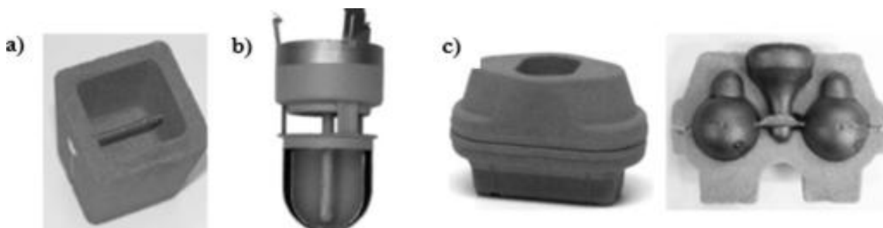
Fig. 5 Cups for thermal analysis; a) Classic open cup with thermocouple; b) Steel cup with two thermocouples in a protective tube; c) AccuVo dual-chamber cup
