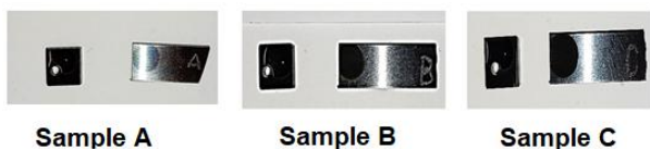
Fig. 16 Test for confirmation of the degree of blackening on individual samples
