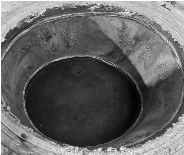
Fig. 10 Bearings after centrifugal casting
