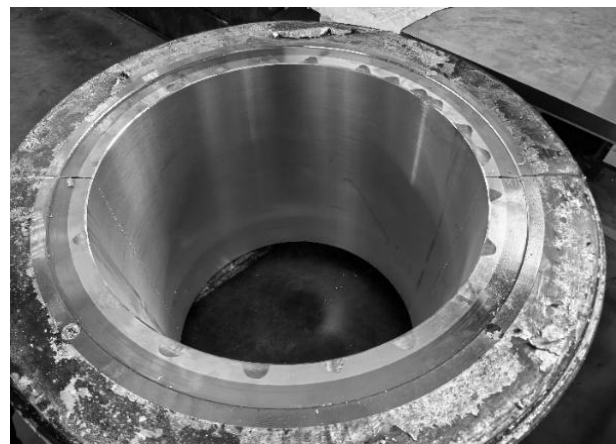
Fig. 11 Thrust bearing products produced by Horizontal Centrifugal Casting
