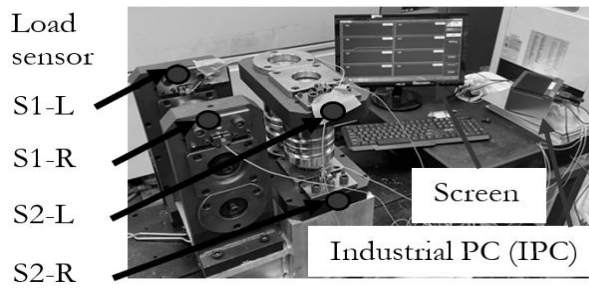
Fig. 11 Rolling mill load sensor installation and display equipment
