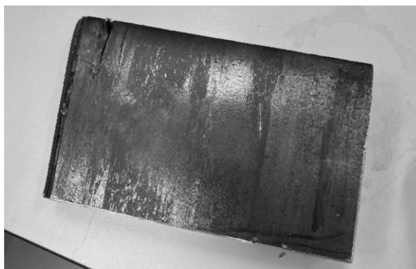
Fig. 2 Sample prepared by hot-rolling
