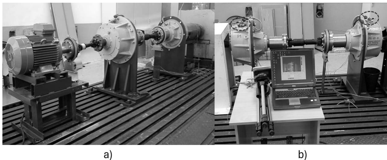
Fig. 1 Test rig assembled in the laboratory of the Department of Design and Machine Elements, University of Žilina; a – final assembly of test rig; b – test rig with highlighted sensor positions
