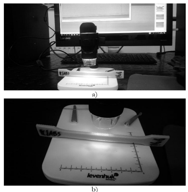
Fig. 5 Example of the thickness measurement for one sample
