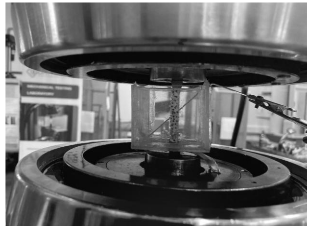
Fig. 1 Close-up of the container with electrolyte and the clamped test specimen
