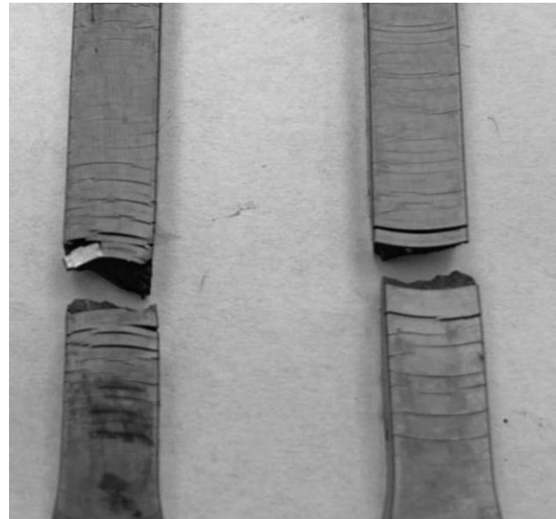
Fig. 9 Close-up of the fracture area of the L80 test specimens
