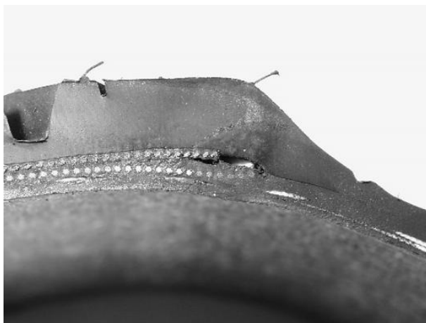
Fig. 35 The cut section of No. 1 casing – Scan 2, Sector 2 – non-serial side – the defect in the shoulder between the buffer linings
