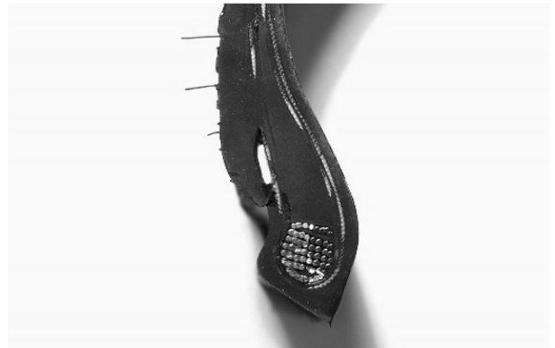
Fig. 37 Cut section of No. 1 casing – Scan 1, Sector 1 – non-serial side – the defect above the bead; The same testing procedure was used for all of the other variants of casings with the same dimensional proportions.
