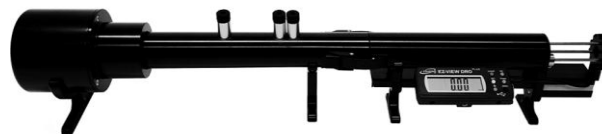
Fig. 8 Impedance tube used for the inverse method [25]
