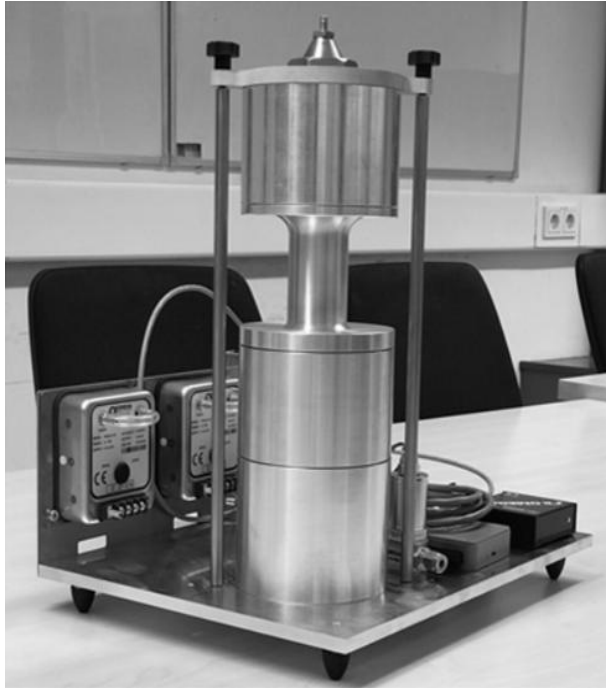
Fig. 5 In-house designed and built quasi-static airflow resistivity meter [5]
