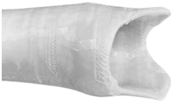
Fig. 9 50% Scale Socket Printing Results
