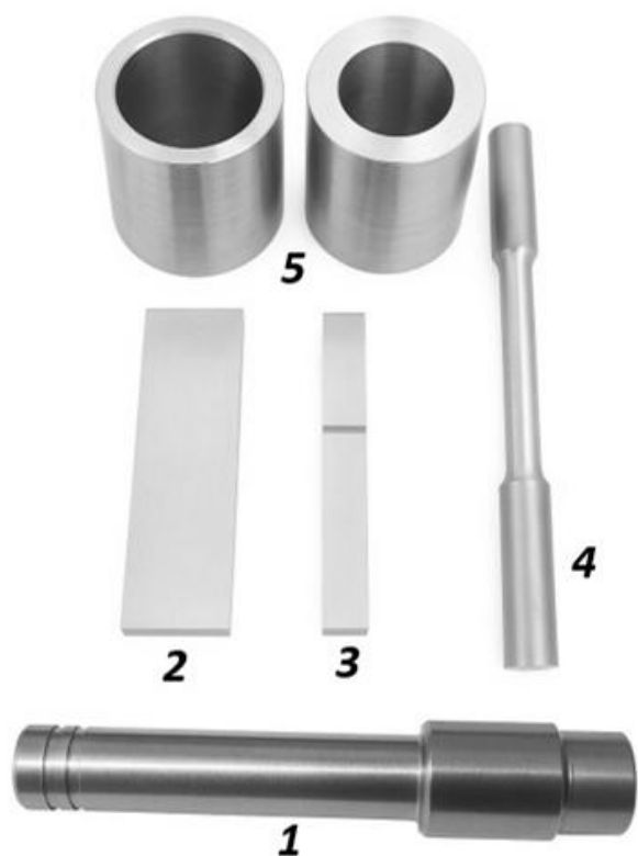
Fig. 3 Types of samples manufactured for the experiment: 1–barrel sample, 2–sample for the Ball-on-Flat test, 3–sample for the impact bending test, 4–sample for the static tensile test, 5–sample for the dimensional stability test
